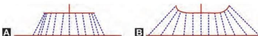
Figs 4.4A and B: Electric fields produced by Flat (A) and (B) Convex electrodes
